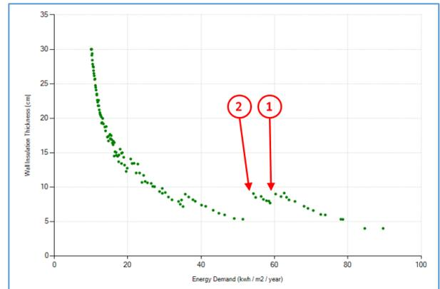
Figure 12: Required wall insulation as a function of the target energy demand
