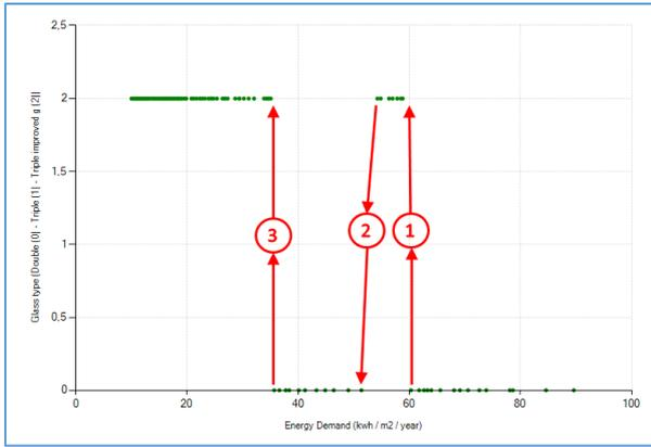
Figure 8: Required glass type as a function of the target energy demand
