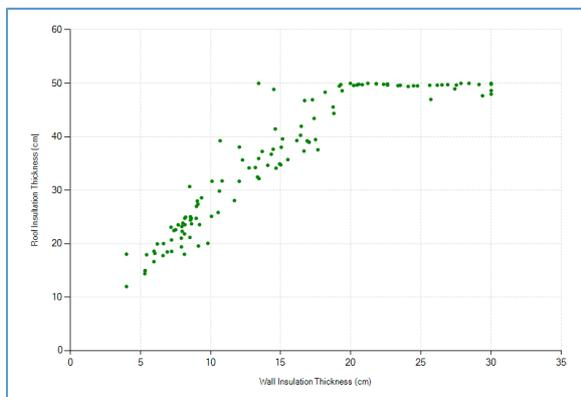
Figure 15: Relation between the optimal Roof Insulation Thickness and the Wall Insulation Thickness
