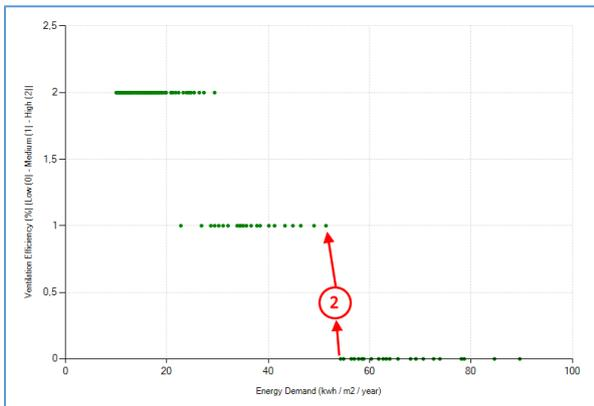
Figure 9: Required ventilation efficiency as a function of the target energy demand
