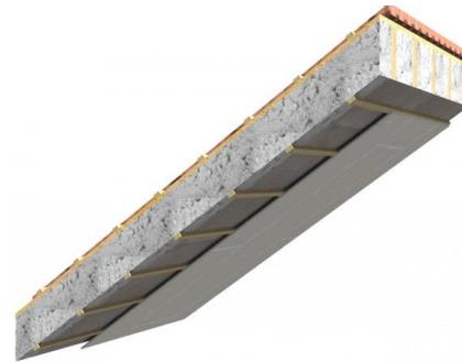
Figure 4: Roof insulated with Cellulose
