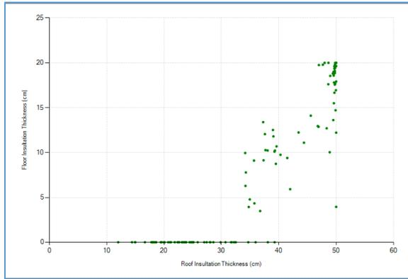
Figure 13: Relation between the optimal Floor Insulation Thickness and the Roof Insulation Thickness
