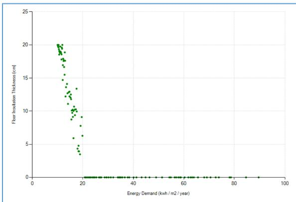
Figure 10: Required floor insulation thickness as a function of the target energy demand
