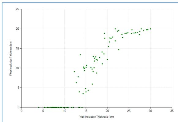
Figure 14: Relation between the optimal Floor Insulation Thickness and the Wall Insulation Thickness
